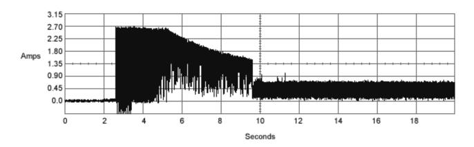
Figure 2. Typical 12V startup and operation current profile
