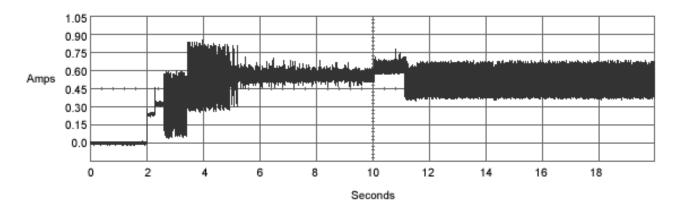
Figure 1. Typical 5V startup and operation current profile
