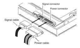
Figure 4. Attaching SATA cabling
