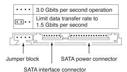
Figure 3. Serial ATA connectors
